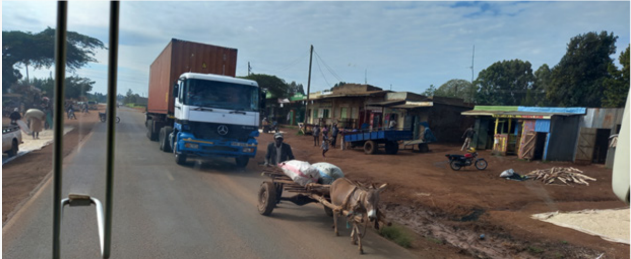
The use of donkeys to transport goods is common along the Eldoret – Kitale road. Since there are no shoulders, the donkey dictates the speed at which motorists move. As traffic grows, this is likely to cause unnecessary jams. Therefore, there is a need for road designers to start planning for non-motorized traffic when designing roads for construction; cyclists, pedestrians, etc.
