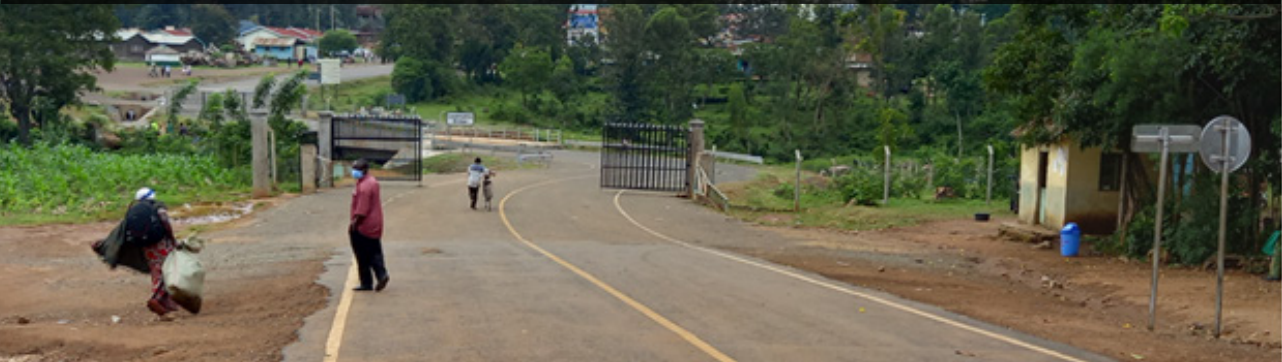
Below: Kenya side of the border offers an opportunity to minimize the curving during an upgrade of the access road from Kenya to the bridge by shifting the access road to the right.
