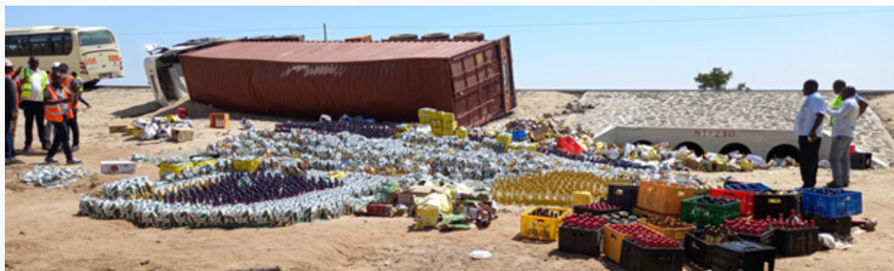
The Lokichar – Lodwar road has very steep edges; any slight veering off the road, the driver may be unable to steer the truck back to the road; thus, the truck is likely to overturn.
