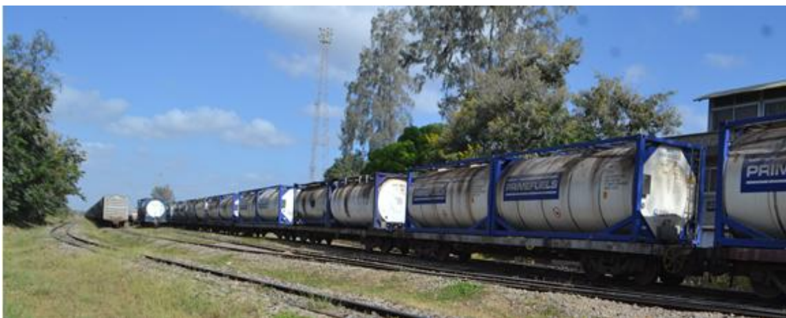
Changamwe MGR Station: A train carrying oil products at Changamwe getting ready for takeoff to Nairobi. Using a single engine, the MGR train can haul between 18 to 22 wagons of oil products to Nairobi.
