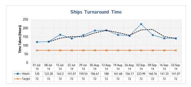
To reduce the ships turnaround time the authorities should focus more on berth time without ignoring the waiting time. It is the component which when reduced can substantially reduce ship turnaround time. The berth time depends on the quantity of cargo a vessel has to load or discharge, the type and characteristics of a vessel, the type of equipment and other resources used at berth.
