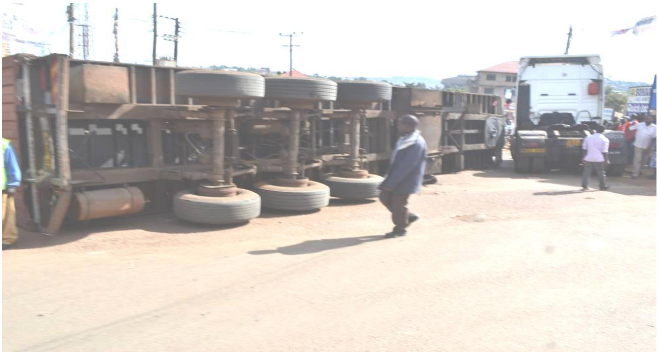
Shifting of cargo in the container was highlighted as one of the likely cause of this accident as the truck was turning off from the main road to Kampala at Bweyogerere.
