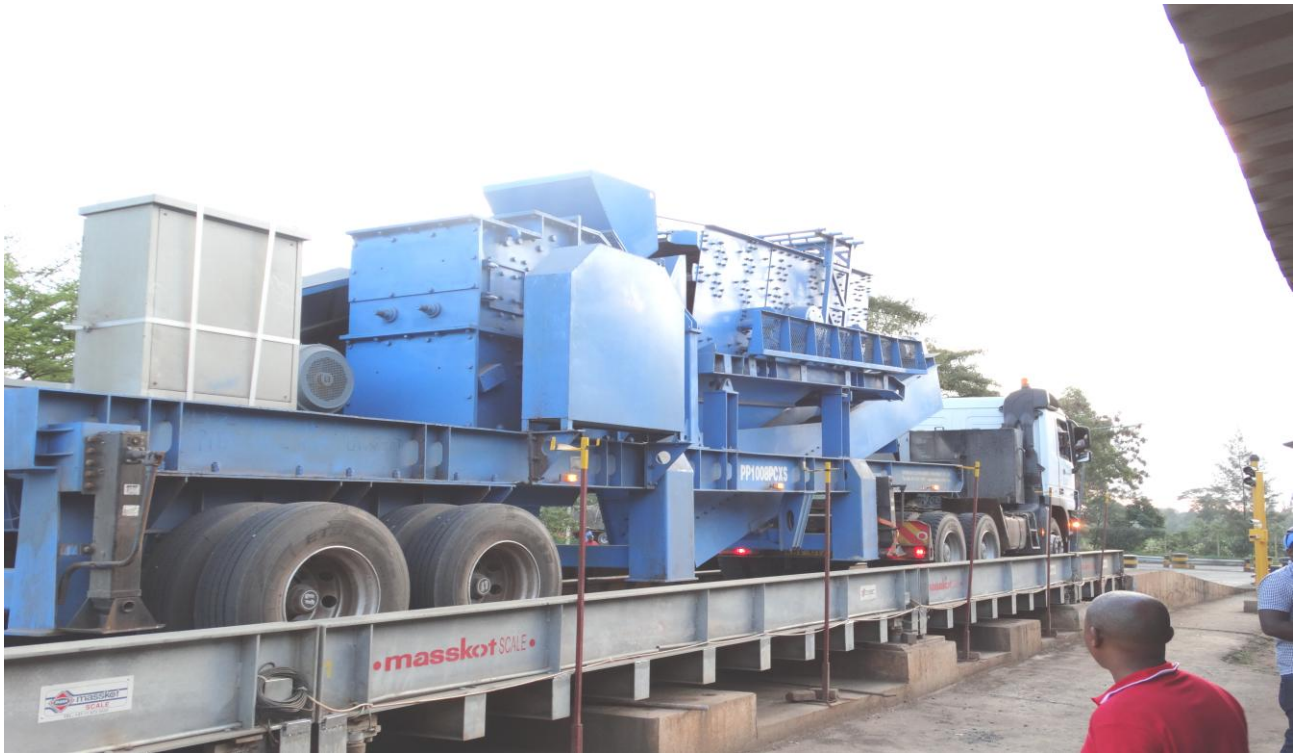
Truck being weighed using a static multi-deck weighing scale at Webuye Weighbridge Station. Trucks carrying abnormal loads are also subjected to vehicle load controls though with special considerations.
