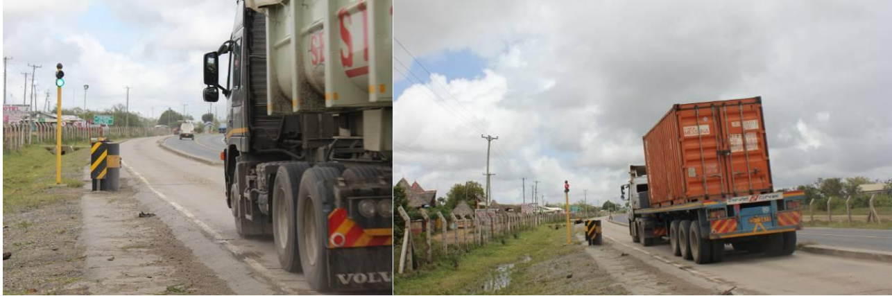
Mariakani HS-WIM; Left: A truck shown a Green Light is compliant and continues on its journey. Right: Truck is shown a Red Light is not compliant, it is diverted to the Static Weighbridge. Currently all the weighbridges in Kenya are being managed by SGS
