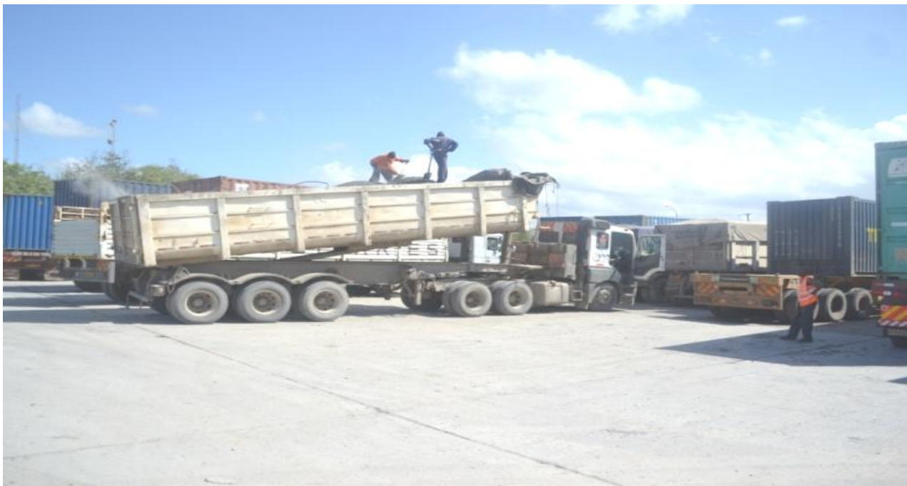
Truckers redistributing cargo at Mariakani weighbridge station: the Survey Team observed that the trucks carrying clinker were the biggest culprits of trucks that complied with GVW limits but not axle load limits, this was attributed to shifting of cargo when the trucks are in motion. How do we minimize shifting of cargo for such trucks?
