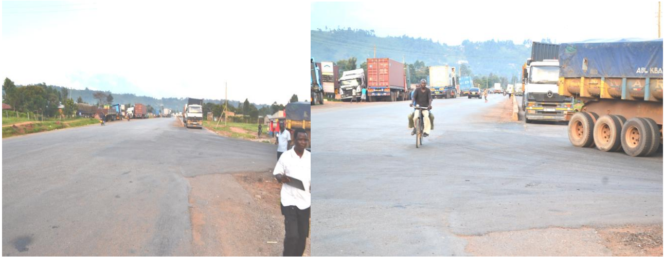
Left: A truck blocks the HS-WIM weighbridge lane as it waits to divert to the Static Weighbridge Scale thereby blocking other vehicles given a green light to proceed on their journeys. Right: Vehicles diverting to the Static weighbridge at Webuye
